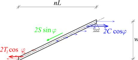
Side-view of the resulting membrane forces under a deflection equal to w
