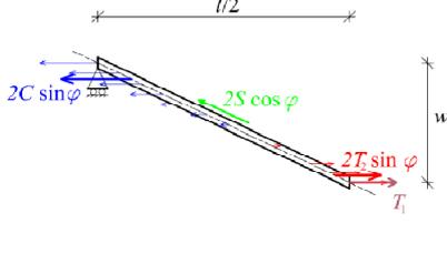
Side-view of the resulting membrane forces under a deflection equal to w
